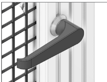
T - Turn Handle and Stop Quarter turn handle with a cam that goes through the door post like a traditional door handle. On the opposite end is a cam that engages with a door stop
