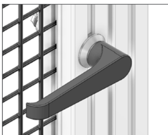
T - Turn Handle and Stop Quarter turn handle with a cam that goes through the door post like a traditional door handle. On the opposite end is a cam that engages with a door stop
